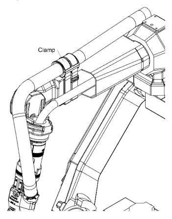
Keep the clamp as far forward on the robot arm as practical while
